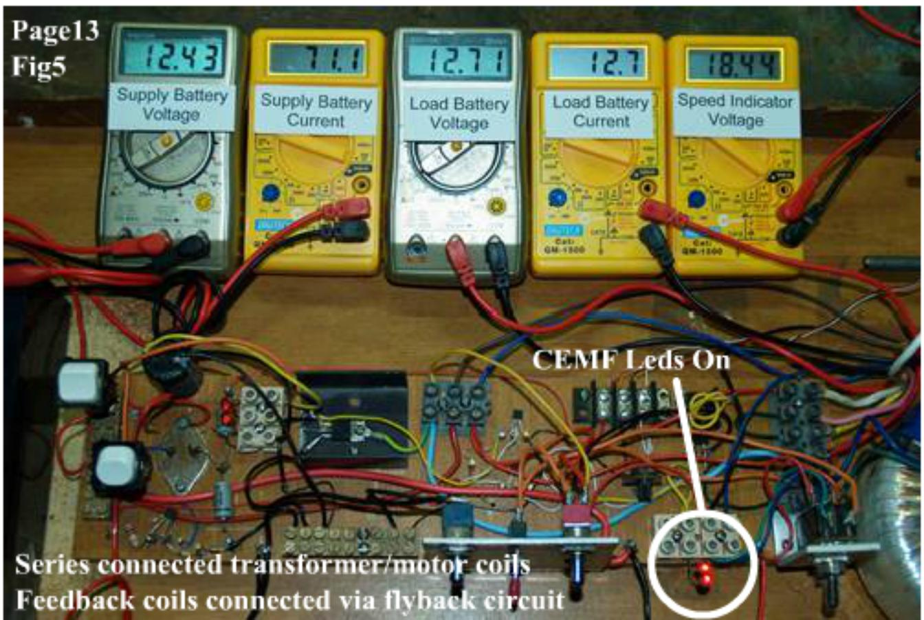
Table 2 below combines the data from table1 with the data from Fig3 and Fig5 above, I can happily say yes to most of my previous questions. With this particular motor's air core coils and transformer arrangement, I can manipulate the cemf more efficiently in order to 1: increase motor speed (running torque), to a greater speed than an unloaded motor. 2: charge a battery load at the same time with cemf . 3: decrease supply current while increasing speed
