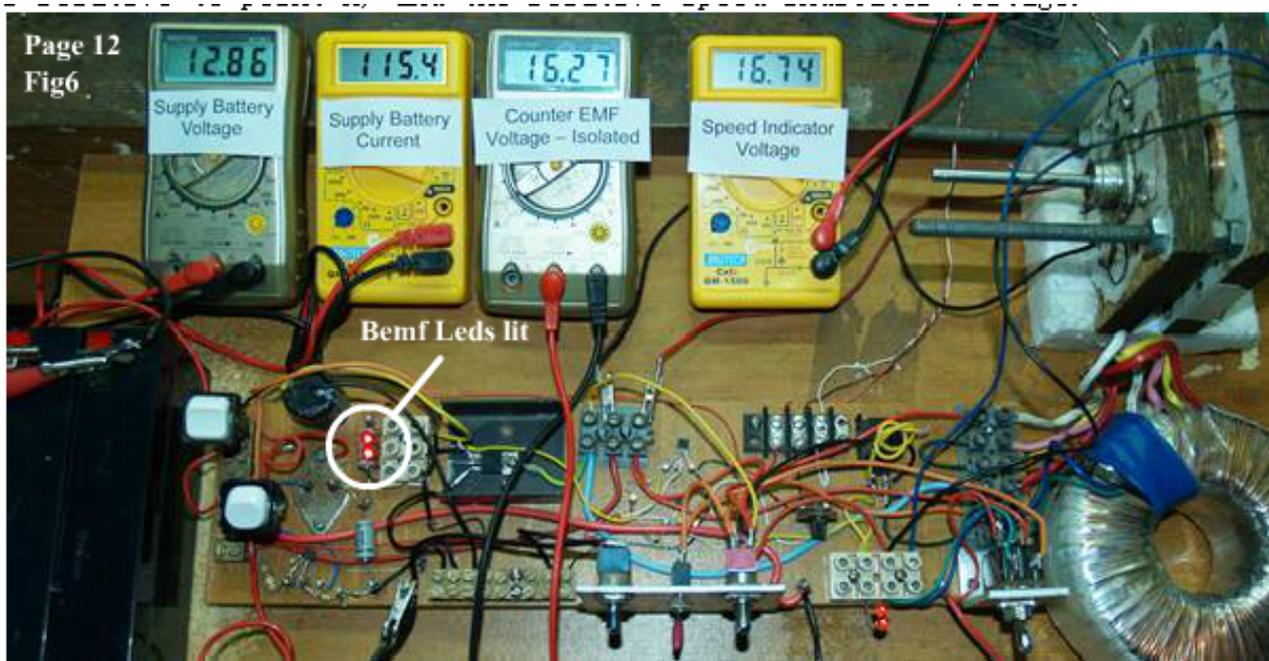
This photo also shows the main switch SW1, SW3 and SW4 operated. There is no attempt to collect or divert the CEMF. The meters show the supply voltage (point B relative to point A), the supply current (in milliamps), the isolated BEMF (Counter emf) voltage across the Leds (point D relative to point B) and the relative speed indicator voltage.
