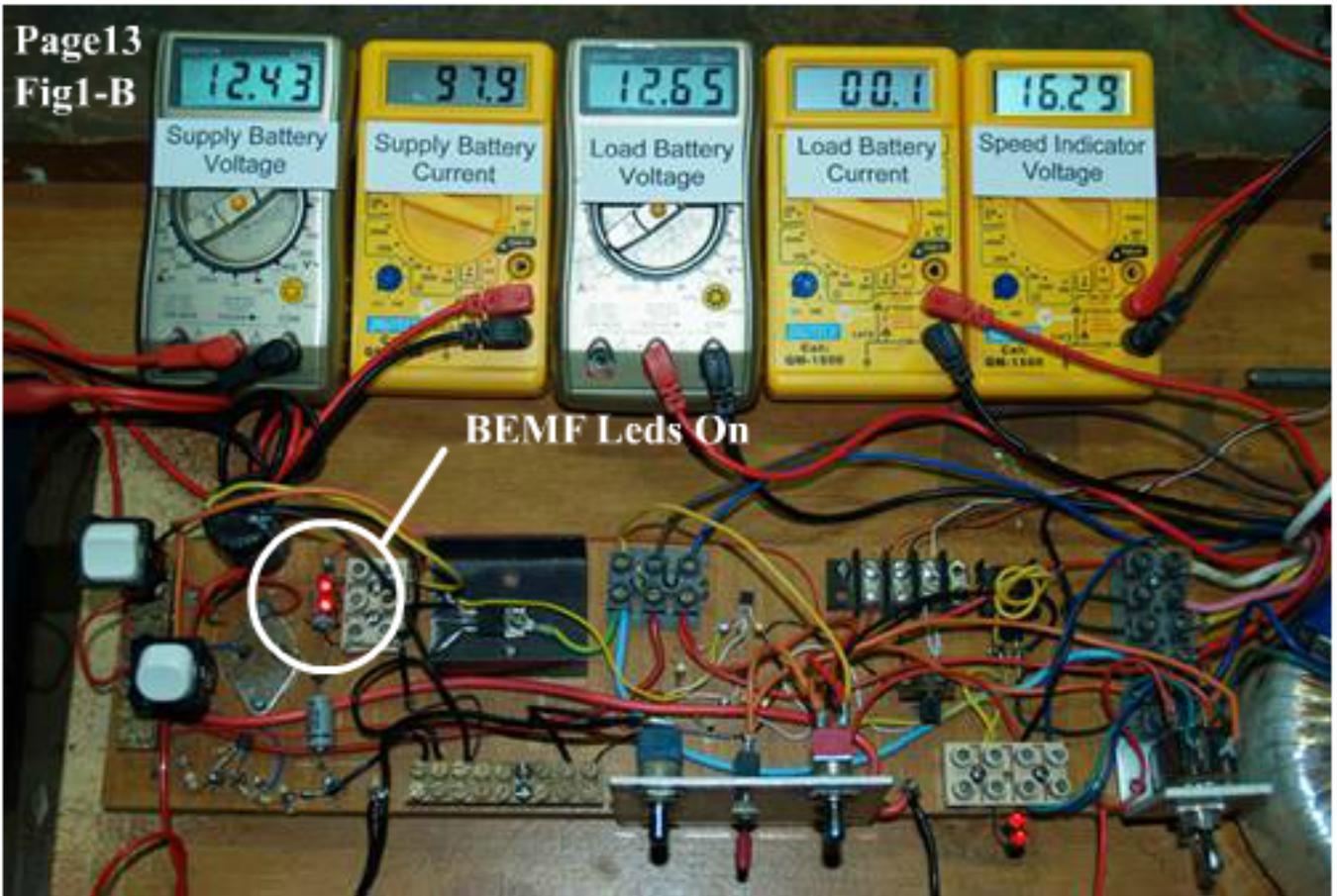
Fig1-C Shows the CEMF (flyback) circuit switched on with CEMF indicator Leds and load battery meters showing current flow and increased battery2 voltage. It also shows a further loss of speed and increased supply current as a result.
