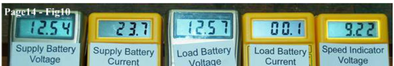
As can be seen by the meter readings, the current is low (23.7ma) but the speed is also very low. The transformer/coils arrangement will only produce its highest motor speed when the cemf circuit is connected and heavily loaded.
