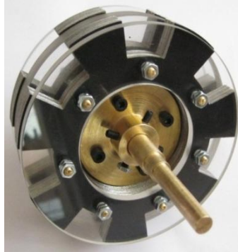
Fig. 3. View of a rotor comprising a shaft, fixing flanges, a magnet enclosure, rotor sections and stratified laminations and side perspex panels with brass bolts to tighten the rotor body
