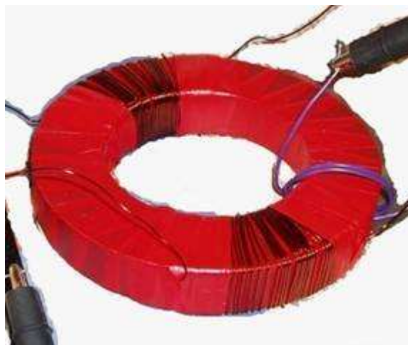
pic1. Two coils wound on ring ferrite core
