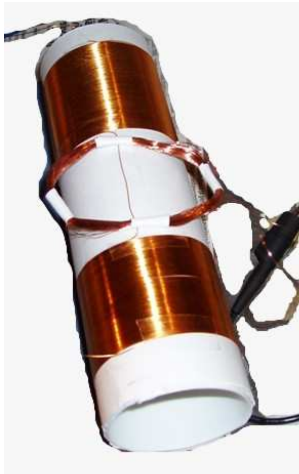
pic6. Different coil used to see if there is a perpendicular magnet field component
