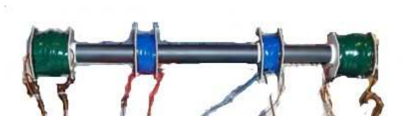
pic4. Two pickup coils placed symmetrically
