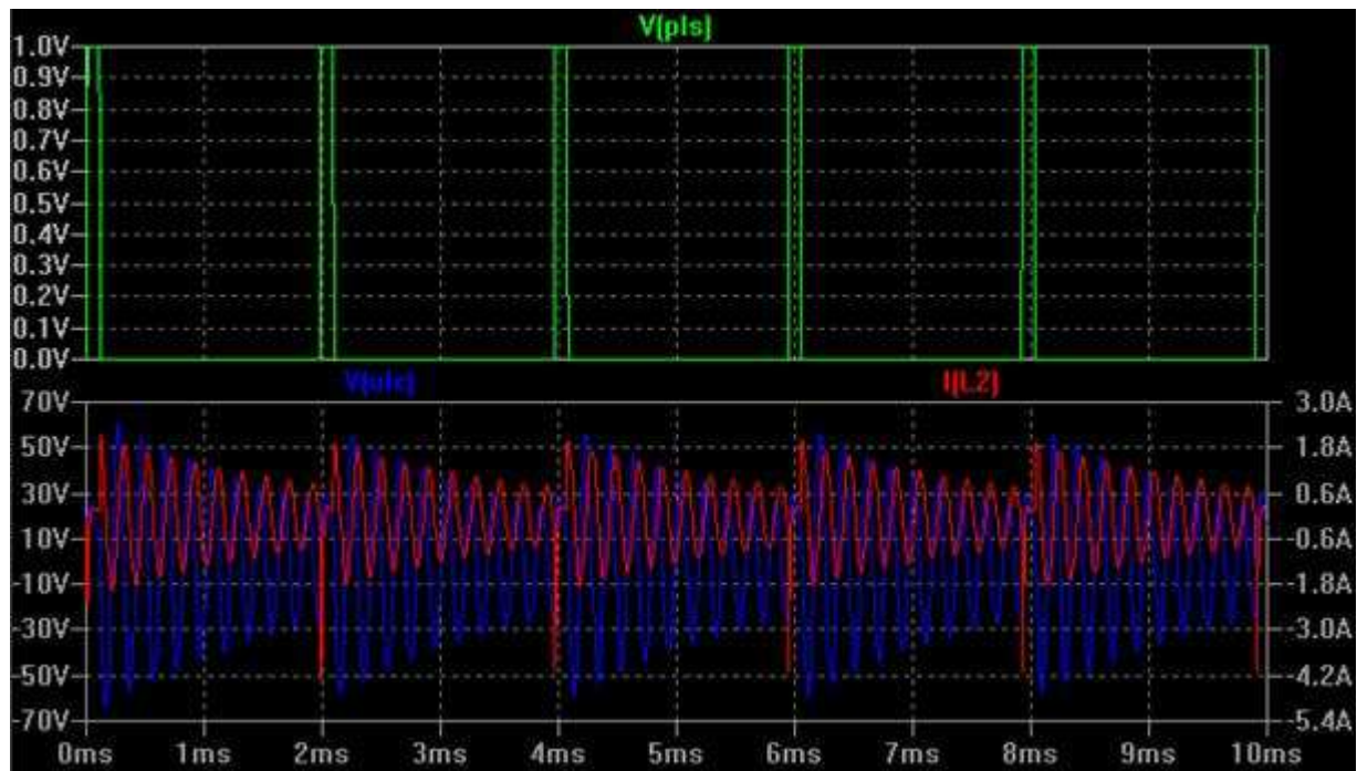
pic3. Simulation (driver frequency 10 times lower than resonance frequency)
