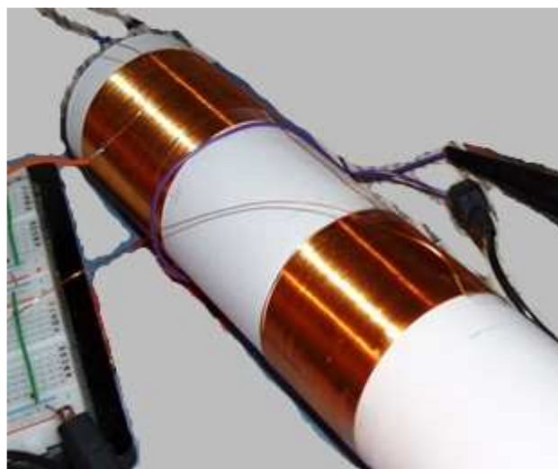
pic2. Bifilar coil type 2
