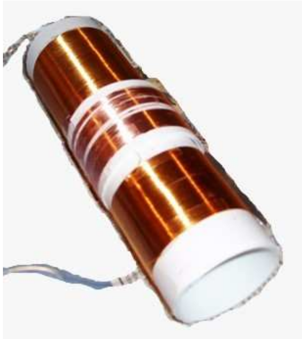
pic8. Two coils wound in opposite direction placed symmetrically relative to 0 point used as pick-up coils
