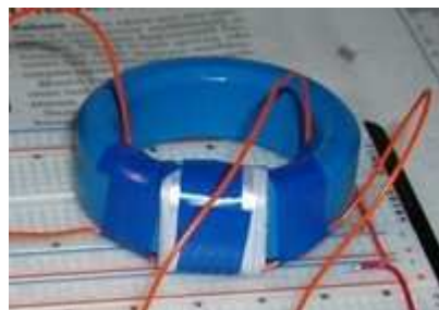
pic1. Coil-capacitor on a ring core (Epcos N30 34x20,5x12,5)
