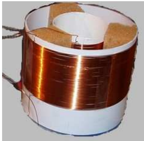
pic1. Bifilar coil type 1
