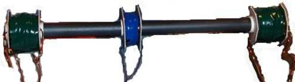
pic2. Moving test coil along the rod
