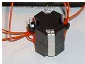
pic1. Coil-cap on RM10 core
